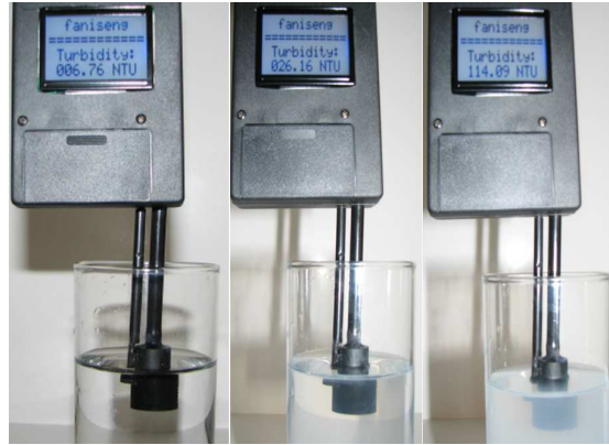
Fig. 7. Demonstration of the turbidity system developed
