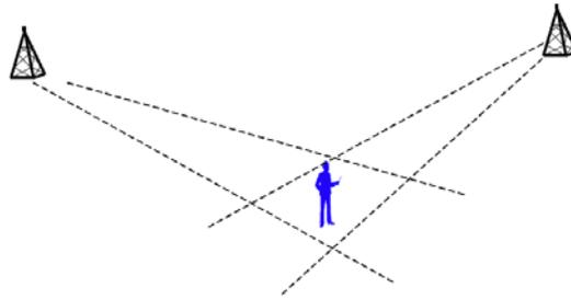
**Figure 1: Positioning with AoA technique.**
