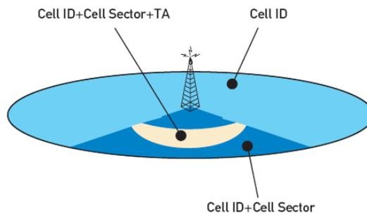
**Figure 2: Positioning with Cell-ID and TA parameter [4].**
