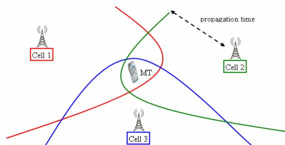
**Figure 3: Positioning based on triangulating ToA measurements.**
