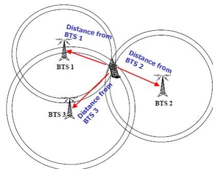
**Figure 4: Positioning with RSS measurements using a propagation model.**
